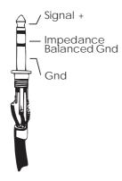
All of the jack socket outputs are impedance balanced. They are on 3-pole a gauge jack sockets, wired as shown on the left and below,. They accept 3-pole 1/4" "A" gauge (TRS) jacks, or 2-pole mono jacks.
